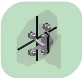
A custom casting connected to a glass fin (mullion) and Planar 902 bolts to façade glass.
