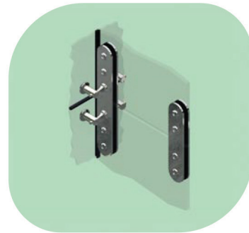
Vertical stainless steel splice plate connecting sections of a glass fin (mullion) together, incorporating Planar 905J fittings.
